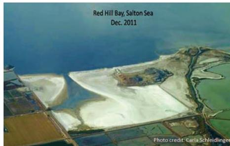
To achieve restoration of Red Hill Bay, water will be pumped from the Alamo River and the Salton Sea and allowed to flow through two 210-acre impoundments. The water will be blended to achieve a target salinity of 20 ppt salt in the first cell and this concentration will increase via evaporation as water flows through the system.
